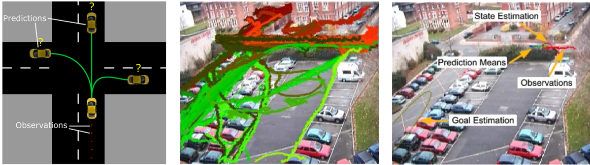
Figure 3: (left) the long-term future motion prediction problem; (center) set of pedestrian trajectories observed on a parking lot; (right) GHMM prediction of the future motion of the currently observed pedestrian (estimation of the state at time t + 10 and of the goal state).
